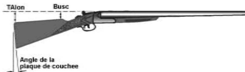
**LA PENTE DE LA CROSSE SE MESURE AU TALON ET AU BUS-**
